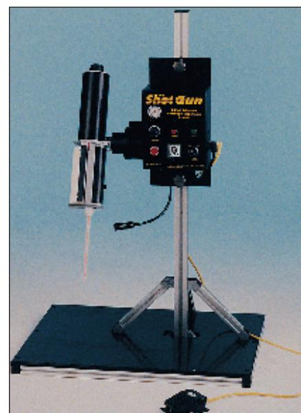
precisely timed shots. Featuring a swivel-gun mount, adjustable height, and adjustable angle rotation for maximum operator productivity, the ShotGun units are mounted on standard, high-density polyethylene worktables equipped with foot-pedal operation for maximum operator comfort.
