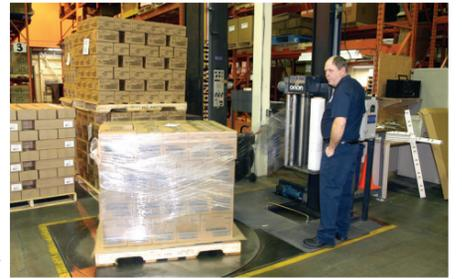
A Trillium employee uses an Orion stretchwrapper to secure cartons of pharmaceuticals to the pallet.
