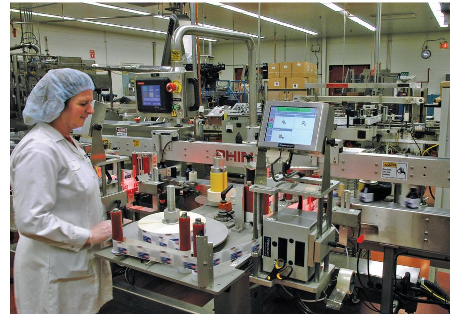
A Trillium employee at the Brockville, Ont. facility watches the custom-built SM 9000 labeling machine, constructed by SPS/PHIN, quickly and accurately apply labels to pharmaceutical packages.
