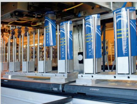
Plastic sleeves are automatically inserted into their nests during a packaging run at the Wilson plant.
