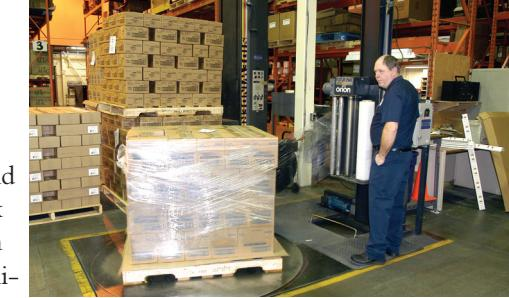
A Trillium employee uses an Orion stretchwrapper to secure cartons of pharmaceuticals to the pallet.
