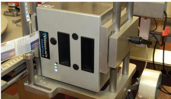
A Videojet Dataflow Plus thermal transfer printer adds coded security data to each label prior to its application to a product.
